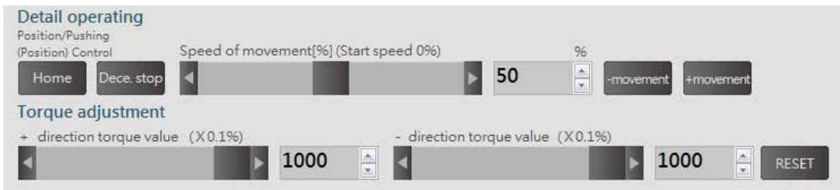
Figure (27) Detailed Operation/ Torque Value Adjustment
